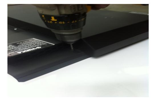
6. YOU WILL NEED TO DRILL THE 2 TOP HOLES WITH A 3.3mm DRILL BIT. THEN FIT THE TOP 2 SCREWS PROVIDED.
