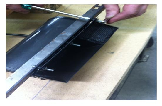
3. FIT THE FAN TO THE BRACKET THROUGH THE 3 PREDRILLED HOLES, WITH THE BOLTS AND NUTS PROVIDED.
