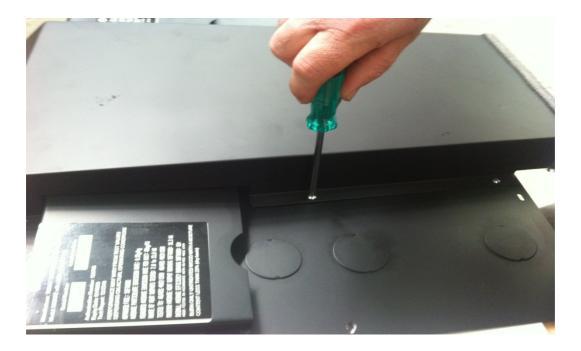
5. ATTACH FAN DUCT TO THE REAR PANEL WITH THE 4 LOWER SCREWS PROVIDED.
