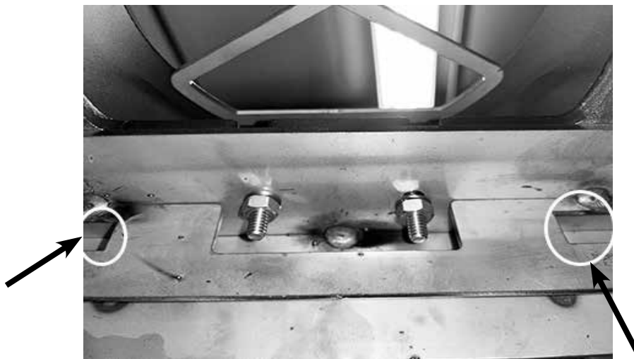
Figure 6. Front mounting slots for Flue Gas Agitator
