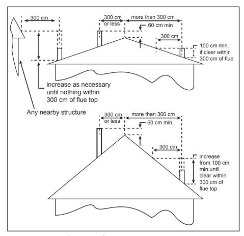
Figure 6. Neo 1.6 Chimney and connector
