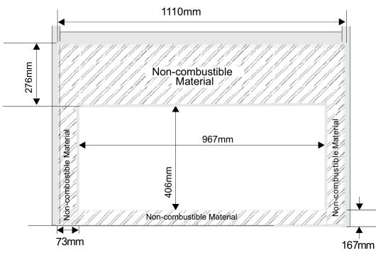
A minimum thickness of 12 mm non-combustible board complant with AS1530-1 and AS1530-3 is required.
