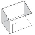
Within a partial enclosure that includes an overhead cover and no more that two walls.
