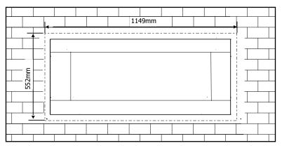
For material such as brick, stone, etc that extend up to 38mm, the minimum opening dimensions noted below must be adhered, when finishing around the faceplate. This is to ensure the removal of the faceplate and for the safe operation of this appliance.
