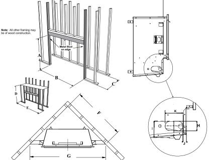
**Important Note:** Two (2) ventilation grills are highly recommended for all enclosures. This is to alleviate moisture and allow for air to circulate. Minimum recommended size: 508 mm<sup>2</sup> ea.
