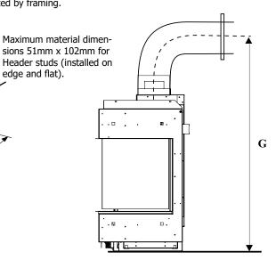
**Note:** This appliance must be installed on a solid surface such as a plywood floor which must be the full width and depth of the appliance.
