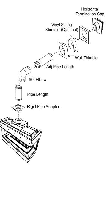
When using Rigid Flue other than Simpson Dura-vent, 3 screws must be used to secure rigid pipe to adaptor.
