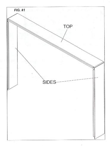
2. The sides sections are attached to the outside of the Top section. At this point you can use screws or silicone to secure the pices together. Fig. #2
