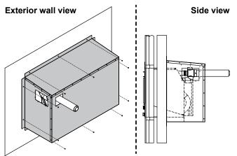
Secure the box assembly to the exterior wall (with appropriate fixings), ensuring that it is both level and symmetrically aligned with the cavity / penetration, the heater support shelf and the appliance.
