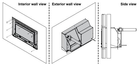
Mount and secure the appliance and connect the flue system in accordance with the OPERATION & INSTALLATION MANUAL, Power Flued Flamefire Gas Space Heater RHFE-951ETR / RHFE-952ER / RHFE-1250ETR / RHFE-1252ER (supplied with the heater) and the INSTALLATION MANUAL, Power Flued Flamefire Space Heater Co-Axial Flue System (supplied with the flue).
