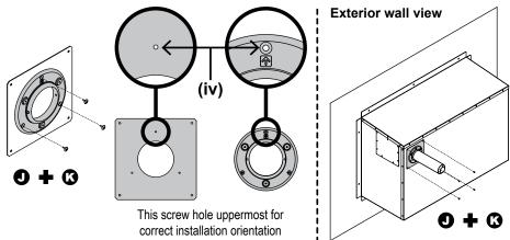
With the screw hole (iv) uppermost, secure the flue terminal wall plate K (supplied with the flue terminal) to the rear (flue) access panel J (SD screws x3), then with the same orientation fit this assembly over the flue pipe and secure it to the box (SD screws x4).
